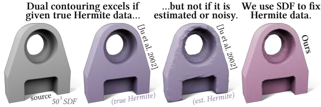
Fig. 5. The outstanding reconstruction quality of classic Dual Contouring depends on having exact Hermite data as input (center left). If approximate (finite difference) estimates are used, quality suffers noticeably (center right). Our method uses the SDF data to optimize for accurate Hermite data, nearly recovering the output quality achieved with exact data (far right).
