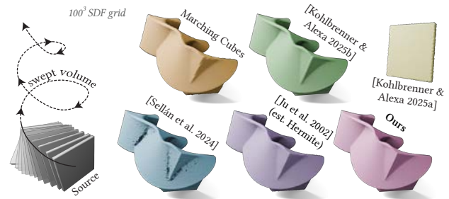
Fig. 18. Sweeping a rigid rectangular plate along a swirling trajectory yields a complex shape with numerous sharp features. Our method produces the best reconstructed mesh compared to competing schemes.
