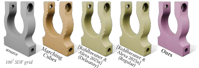
“Marching” (cubes/tetrahedra) methods cannot recover sharp features, unless these are aligned with their volumetric discretization
