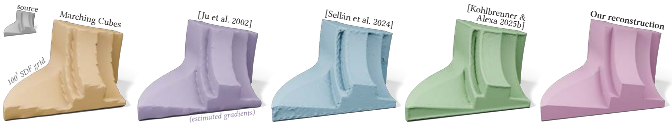
Fig. 1. We propose an algorithm to reconstruct surfaces with sharp features from discrete signed distance data without the need for gradient information.
